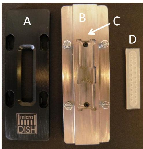
**Figure 4.** Disassembled Flow Cell; A. Top part (= lid); B. Bottom part with the liquid channel and space for the insert; C. Sealing rubber; D. Porous aluminium oxide and glass insert. *Photo: H. Dietrich.*
