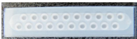
Figure 2. MD Flow Cell insert: consisting of that is a sandwich construction build-up of glass-PAO-glass. The insert shown has 20 wells with a top diameter of 2 mm. Photo: H. Dietrich.
