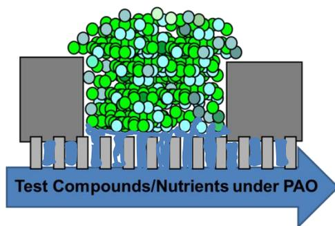
**Figure 3.** Illustration of the MD Flow Cell principle. One compartment (= well) is shown (grey large bars). The test fluid flows underneath the PAO and is sucked by capillary forces upwards inside each well. Microorganisms are depicted as blue/green circles.
