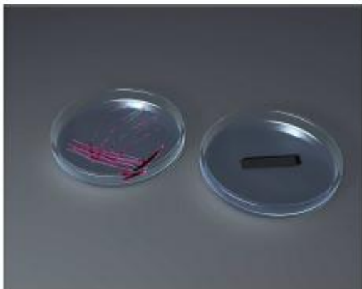
Figure 1. View of a MDCC20 chip lying on top of a Petri dish (right) allowing multiplexed culturing compared with conventional culturing of a single strain on agar (left).
